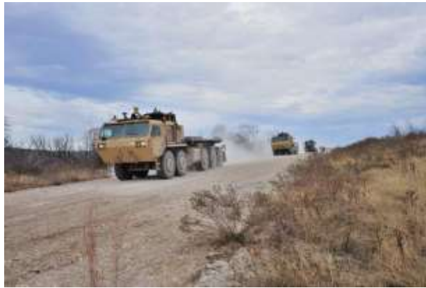
A convoy of PLS and M915 Army trucks gets a test at Fort Hood, Texas. Testers were sometimes in the driver seats, but the vehicles were operated robotically.
